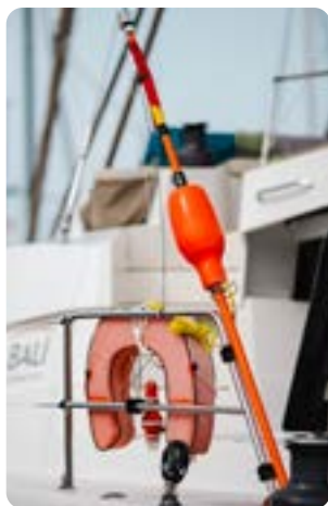
Lifebuoy & danbuoy - L: inflatable, R: permanent buoyancy
