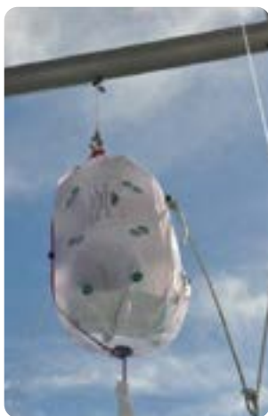
Radar reflectors - L: inflatable & R: octahedral
