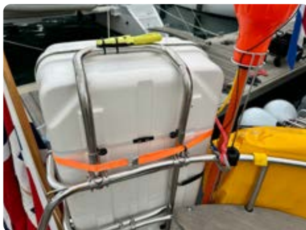
Safety knife stored with the liferaft to cut the painter
