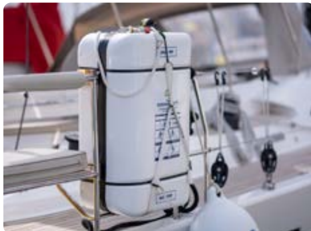
Canister liferaft with a hydrostatic release unit
