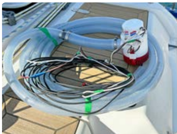
Emergency electrical pump with 233 litre/minute capacity
