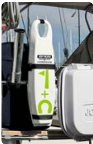
Lifebuoy & danbuoy - L: inflatable, R: permanent buoyancy
