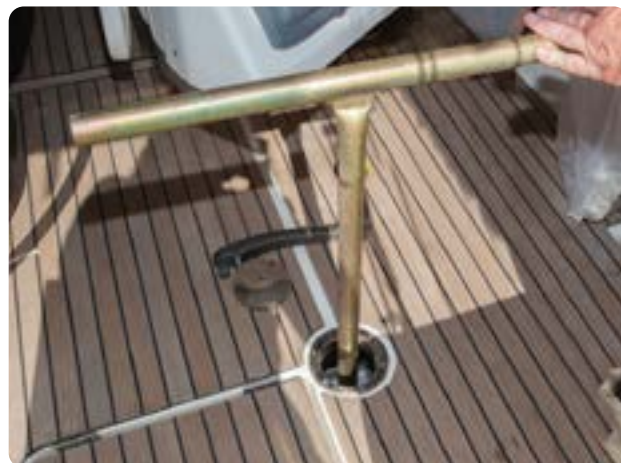
Emergency tiller on a Beneteau Oceanis 46
