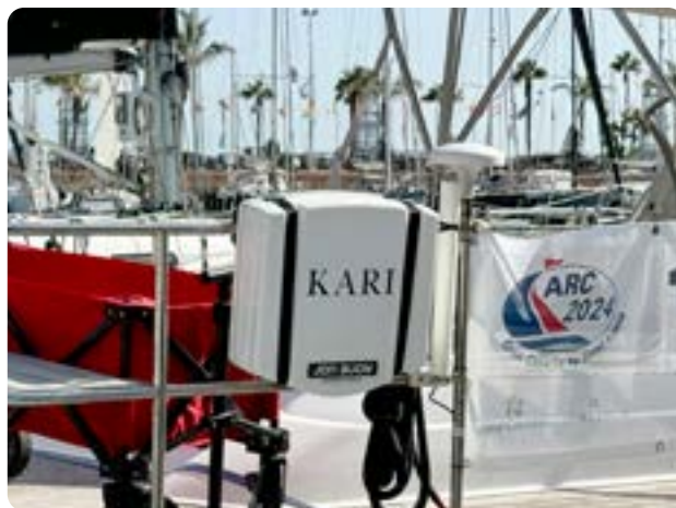
A Jon Buoy MOB module mounted on the aft rail
