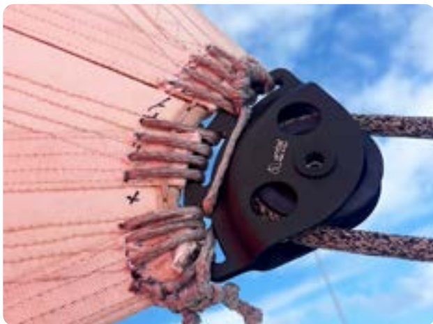
Glemm's torn-out main clew. Credit Guido Rivolta
