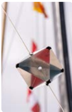
Radar reflectors - L: inflatable & R: octahedral
