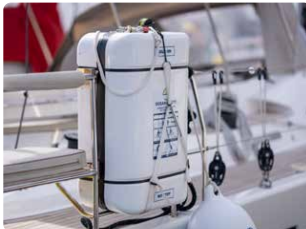
Canister liferaft with a hydrostatic release unit
