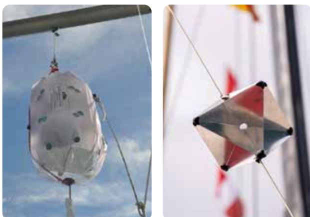
Radar reflectors - L: inflatable & R: octahedral
