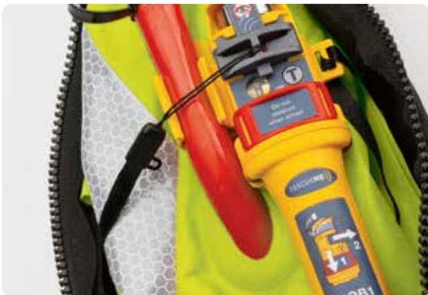
Ocean Signal MOB1 AIS beacon fitted inside a lifejacket
