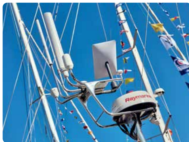
Starlink, radar, AIS and satcoms antennas
