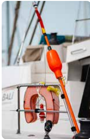
Lifebuoy & danbuoy - L: inflatable, R: permanent buoyancy
