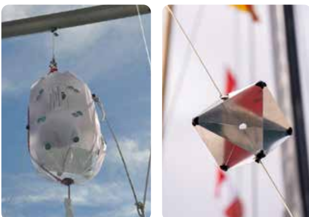
Radar reflectors - L: inflatable & R: octahedral
