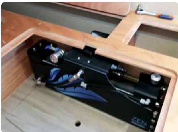
Schenker Zen 30 installed under a bunk
