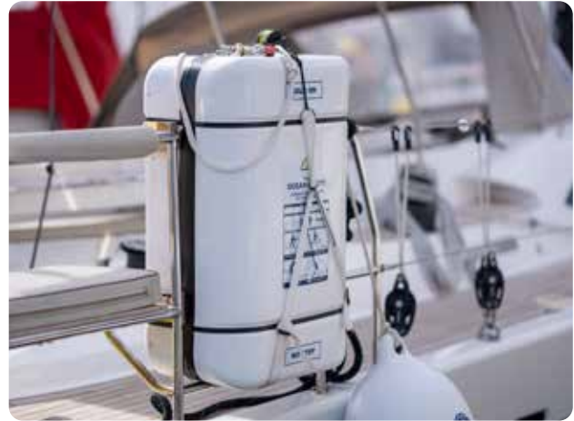
Canister liferaft with a hydrostatic release unit
