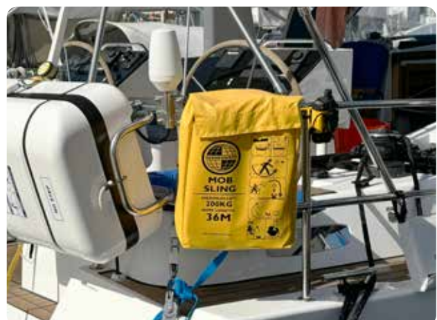
A recovery sling mounted on the aft rail
