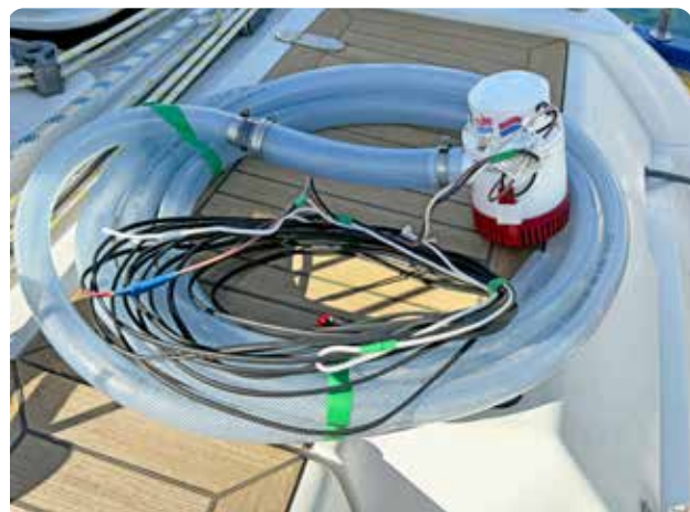
Emergency electrical pump with 233 litre/minute capacity
