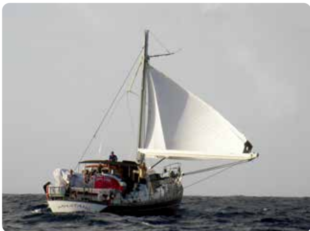
C&N 83 Mustang made an effective jury rig
