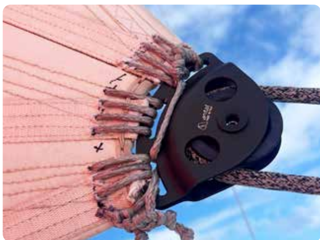
Glemm's torn-out main clew. Credit Guido Rivolta
