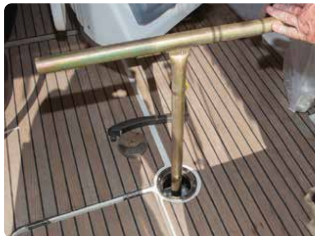
Emergency tiller on a Beneteau Oceanis 46
