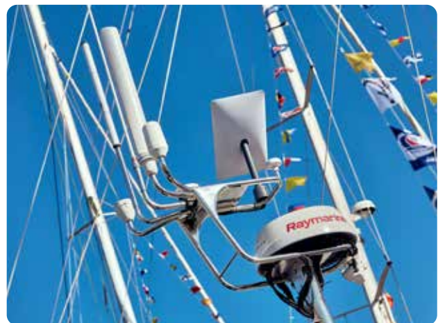
Starlink, radar, AIS and satcoms antennas
