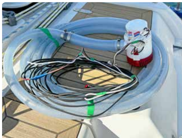
Emergency electrical pump with 233 litre/minute capacity
