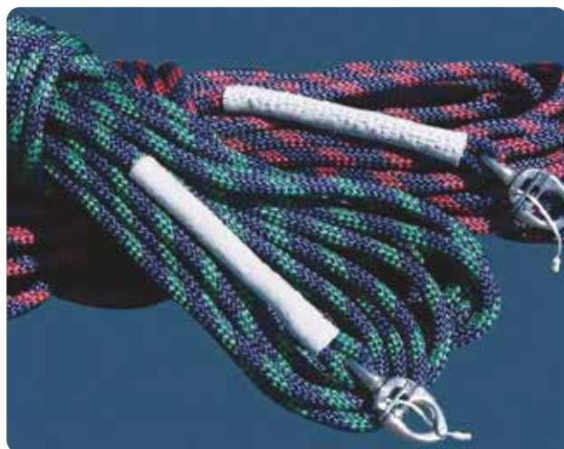
Chafe protection on spinnaker sheets
